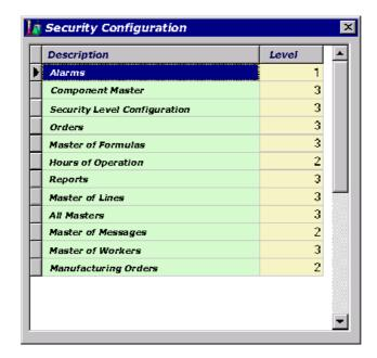
Set up access level on menu option "Security Level Setting".
