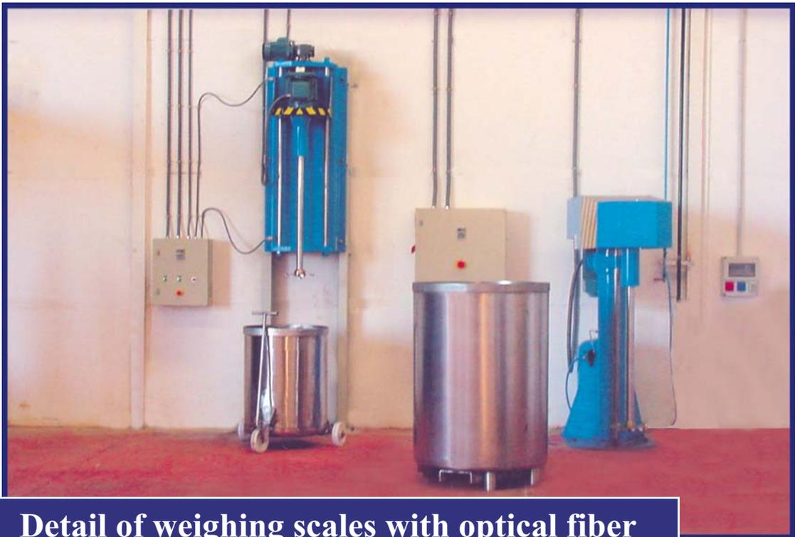
**Detail of weighing scales with optical fiber**
