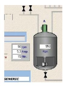
System analogue variables (rpm, amperes, weight) appear in digital values on the body of respective components.
