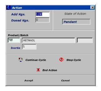
For example, clicking on "Add solvent", opens a window where amount of product and product data (component, batch, inertia) can be selected. State of action is also indicated: done, in process, interrupted. Likewise, other actions can be selected: Continue process, Stop process, End action.
