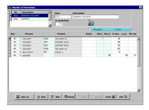
On the lower side of the screen, there are buttons to **Create** new formulas, **Edit** formulas, **Delete**, **Delete line**, **Print** and **Save as**. You can create a new formula making changes on an existing one and changing the name clinking on **Save as**.
