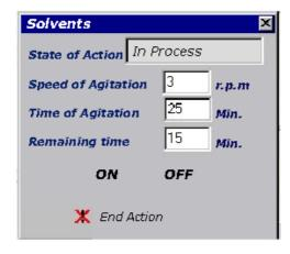
State of action field indicates state of agitation process: In process, Interrupted or Finished. Action must be finished to change rpm and time of agitation.
