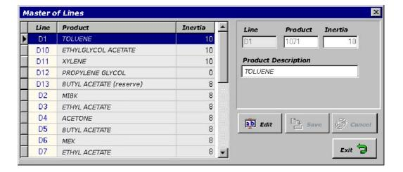
In this master, you can also enter inertia data in kg. used to close the valve in order to compensate pipe inertia.
