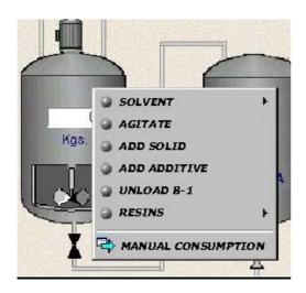
To make an action, right click on appropriate reactor opens a window with different options. Click on action desired to open a new pop-up window to enter conditions of action.
